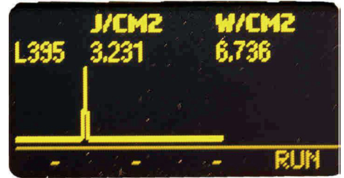
Graphic Mode-collected numerical values and graph of normalized irradiance.
