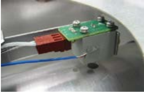
An EIT Compact Sensor mounted behind a UV reflector can provide continuous information on the lamp condition.
