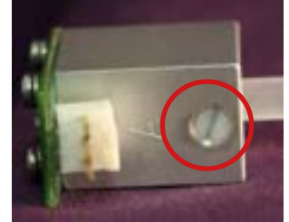
Right: Close up of set screw holding the Quartz Rod into a CS-1 Sensor housing
